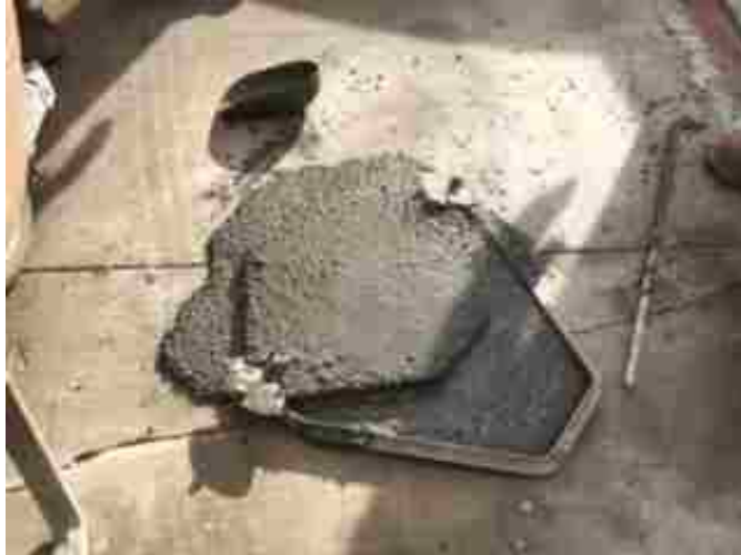
Figure 8- “Invalid” Slump Test Due to Very High Slump Flow
