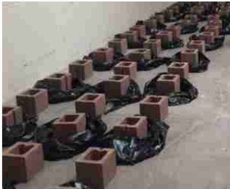
Figure 2- Blocks laid in order for prism construction
